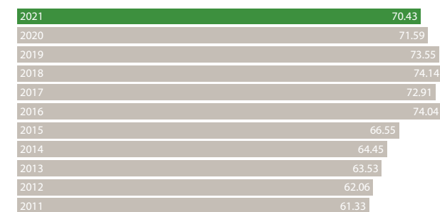
Comprehensive Energy Consumption per Ton of Cement from 2011 to 2021 Unit: kg of standard coal/ton
